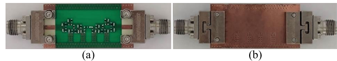
Fig. 17. Photographs of the fabricated reflectionless BPF. (a) Top view. (b) Bottom view.
