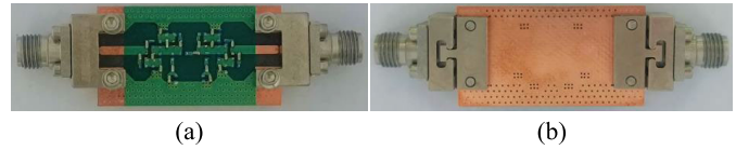
Fig. 21. Photographs of the fabricated reflectionless wideband BPF. (a) Top view. (b) Bottom view.
