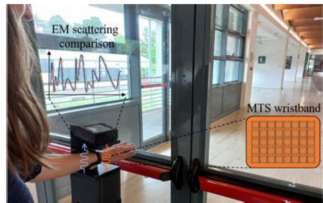
Fig. 1. Representation of an access control application with a device mockup of the proposed MW-based biometric recognition system and the exploitation of the designed MTS wristband.
