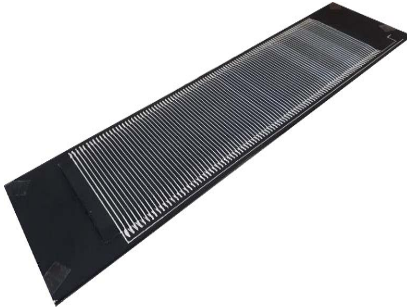
Fig. 3. Photograph of one of the four tangential H-coils of 300 mm × 85 mm × 1 mm effective size, as manufactured by a semi-automatic “3-D/2-D assembler.”
