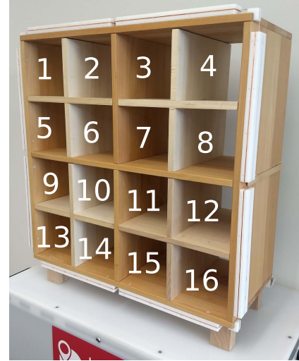
Fig. 8. Wooden shelf with 16 compartments surrounded by an exciter wire and eight pickup coils around its square front. The exciter wire goes through the white plastic elements and the pickup coils are wound around them.
