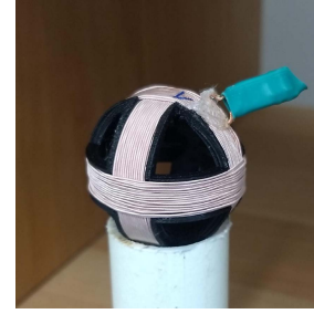
Fig. 9. 3-D coil consisting of three orthogonal identically wound circular coils which are tuned to resonance by capacitors (covered by a turquoise heat shrink tubing).
