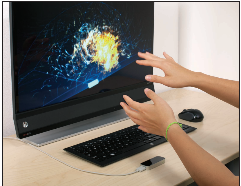
Figure 1. The Leap Motion Controller (foreground) lets users control computers by moving their hands, fingers, finger joints, or various objects.
