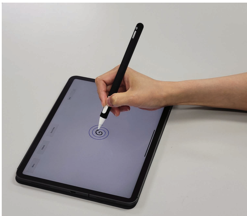
FIGURE 2. The tablet-based application using hand drawing for CTS screening. Participants drew a spiral of 4 cm in diameter using a stylus. The tablet measured the stylus trajectory and pressure of the stylus tip over time.
