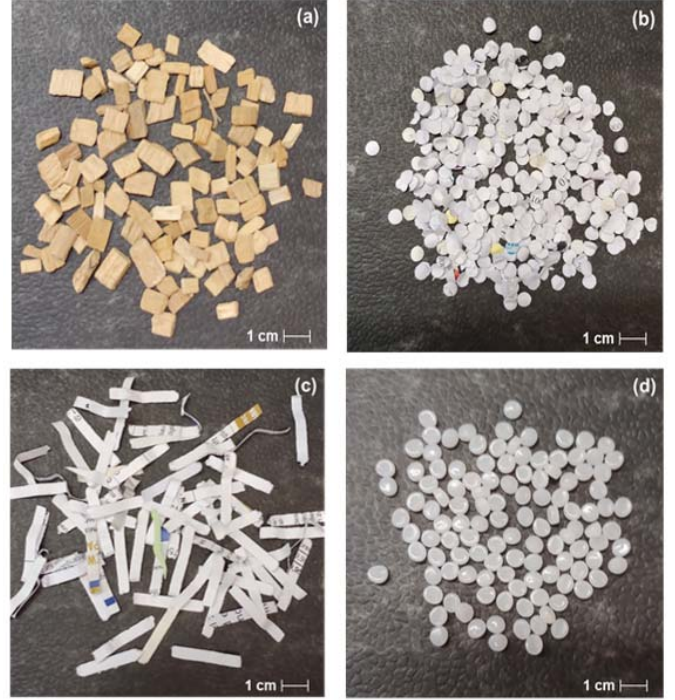
Fig. 15. Various investigated fuel fractions. (a) Wood chips. (b) Confetti. (c) Paper shreds. (d) PE granules.
