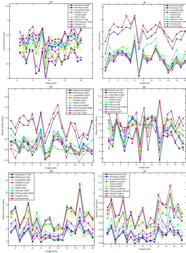
Fig. 12. Quantitative comparison results of CLF-Net and nine state-of-the-art methods on 20 images from the RoadScene dataset. Six metrics are used for comparison: EN, MI, VIF, SD, AG, and SF. The compared methods are DenseFuse, RFN-Nest, FusionGAN, GANMcC, IFCNN, PMGI, U2Fusion, STDFusionNet, IFSepR, and CLF-Net.
