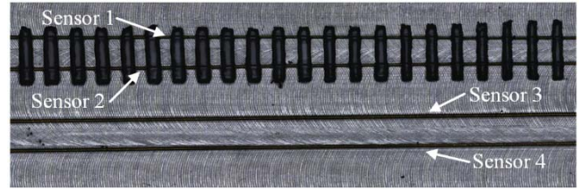
Fig. 9. Section of a metal sample containing two periodic and two randomly perturbed sensors. The sample is coated using a transparent coating.
