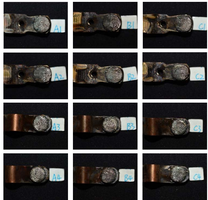
Fig. 2. Contact erosion after an ac-4 test contact carrier, contacting alloy.
