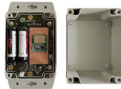
Fig. 5. Customized D-shuttle radiation sensor soldered onto the intermediate board and connected to the communication board. The device is hosted in an IP67 plastic box.
