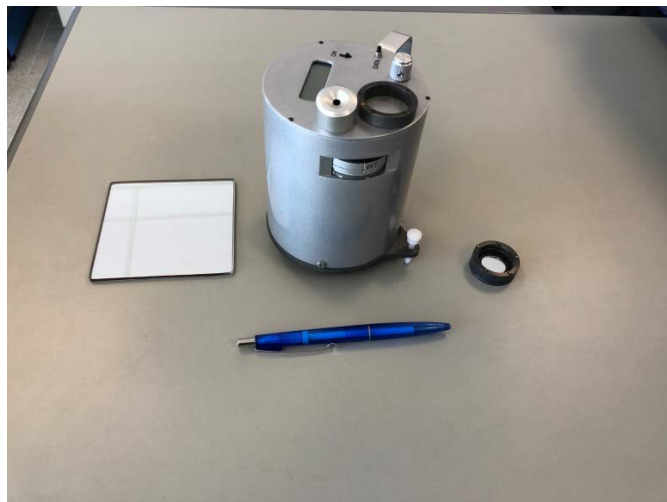
Fig. 7. Different reference mirrors used for this experiment: ext4 (left) and internal reference mirror (right).
