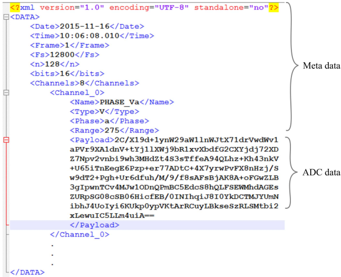
Fig. 9. XML data format used for communication of sample data between DAQ unit and signal processing unit. Sample data is expressed in base64 so that it may be represented as ASCII characters.
