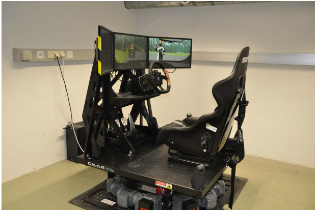
Fig. 1. Driving simulator platform used for the experiments with the capacitive sensor equipped steering wheel [4].
