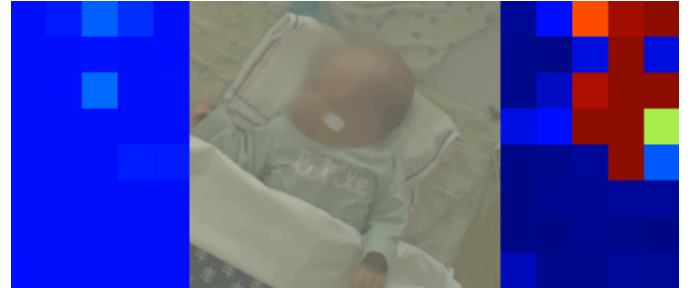
Fig. 8. Visual example of movement and location monitoring using 2-D outputs of the fiber mat. The left heat map shows the movement detected by the specific node. The right heat map shows the raw signal of each node.
