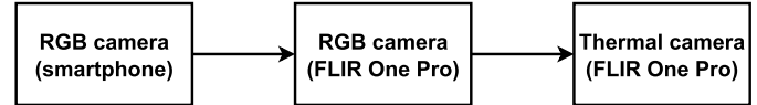
Fig. 3. Cross-spectral mapping of ROI is a two-step process: in the first step, the ROI is mapped from RGB video to FLIR RGB video, and in the second step, the ROI is again mapped from FLIR RGB video to thermal video.
