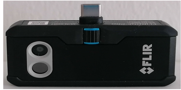
Fig. 2. FLIR One Pro camera device consists of two cameras: an RGB camera (top) and a thermal camera (bottom).
