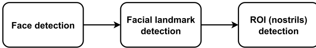
Fig. 7. Method for the detection of nostrils consists of three steps: 1) detection of face; 2) detection of facial landmarks around the nostrils; and 3) detection of ROI based on the facial landmarks.
