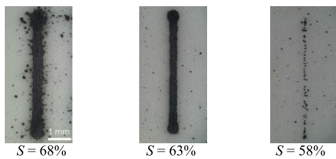
Fig. 8. Effects of Stroke ( S ) on the deposition of Ti 3 C 2 T x . ( Close Volts = 115 V, Pulse = 0.50 ms, Close = 0.4 ms, and Pressure = 0.4 bar).
