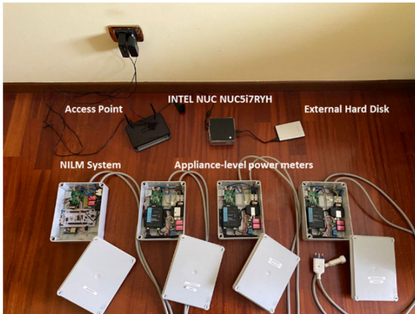
Fig. 8. Overall system installed in the two houses observed during the test phase.
