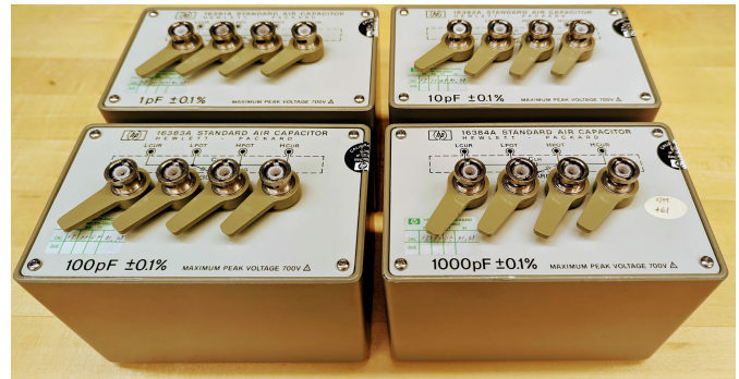
Fig. 1. Commercial set of four standard air capacitors with nominal values of 1, 10, 100, and 1000 pF.
