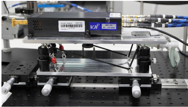
Fig. 4. Alignment system for VNA frequency extenders.
