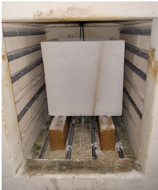
Fig. 8. Refractory container with a sample of limestones in a ceramic kiln.
