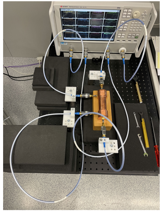
Fig. 2. Measurement setup used for the VNA measurements.
