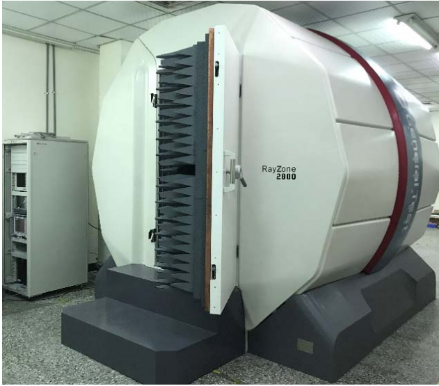
Fig. 9. Validation system mainly includes an anechoic chamber and a BS emulator (integrating a channel emulator inside).
