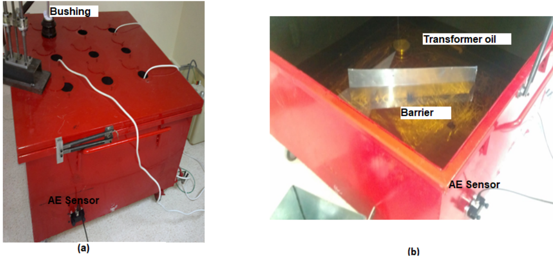
Fig. 3. Overall system setup. (a) Transformer tank system. (b) Location of the barrier inside the transformer tank model.
