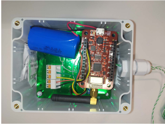
Fig. 11. Photographs of the IoT sensor module prototype used for depth measurement.
