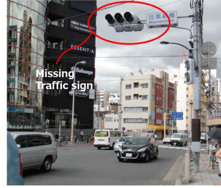
Fig. 4. Missing pulse-controlled LED traffic light caused by electrical shutter, which is caused by the same mechanism as the LED flicker.
