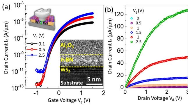
Fig. 4. (a) Transfer characteristics  $I_d$ - $V_g$  and (b) output characteristics  $I_d$ - $V_d$  of a solitary GSG-heterojunction-FET (GSG-HFET). The upper inset in (a) shows the structure of the separately fabricated GSG-HFET, and lower inset in (a) shows TEM image of the gate-stack of the transistor component, verifying the thicknesses of  $\text{WS}_2$  channel,  $h\text{-BN}$  and  $\text{Al}_2\text{O}_3$  dual-layer gate dielectrics to be  $\sim 1$ , 5, and 5 nm, respectively.
