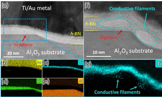
Fig. 5. (a) Cross-sectional TEM image of RRAM component. The energy dispersive X-ray (EDX) analyses from blue rectangular region confirm the (b) Au, (c) Ti, (d) B, and (e) Al elements in corresponding layers. (f) Two CFs are clearly visible around the graphene edge. (g) EDX element mappings of Ti uncovers that these filaments are attributed to Ti.
