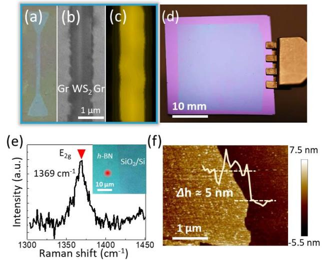
**Fig. 3.** (a) Optical image, (b) SEM image, and (c) Raman mapping of a GSG heterostructure fabricated through area-selective CVD technique. (d) Photograph of the wafer scale CVD *h*-BN film on SiO<sub>2</sub>/Si substrate. (e) Raman spectrum of *h*-BN film shows a characteristic peak at 1369 cm<sup>-1</sup> corresponding to the  $E_{2g}$  vibration mode of the hexagonal B-N bonds. (f) AFM image of the *h*-BN film on SiO<sub>2</sub>/Si substrate shows the thickness of *h*-BN film to be ~5 nm.
