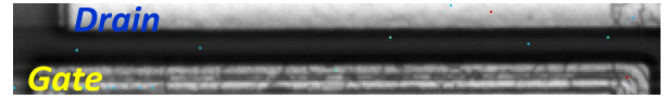
Fig. 9. EL signal detected during the pulsed measurements in soft switching (DGD = 3.3 \mu\text{s} ) after the evaluation in hard switching. Low EL intensity clarifies the absence of permanent degradation.
