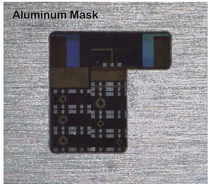
Fig. 9. Micrograph for the whole chip with aluminum mask.
