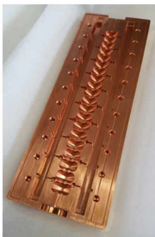
Fig. 1. One half of distributed coupling linac designed at SLAC. Each of the 20 cells in this linac is about 13.1 mm long.
