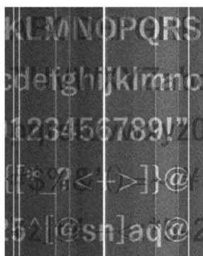
Fig. 6. Reconstructed image with the conventional RVSIA. Because of the multiple screen information contained in the leaked EM wave, the pixels of the left and right sides of the screen information are overlapping. From this reconstructed image, it is difficult to recognize all characters.
