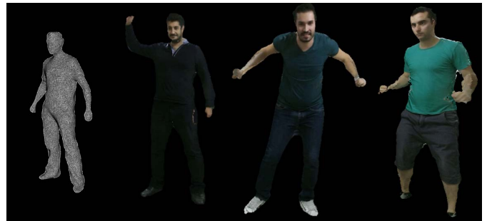
Fig. 2. 3D reconstructions produced by the studied 3D media tele-immersive pipeline. On the leftmost the pure geometry output is shown, while on its right the remaining three 3D reconstructions depict fully textured outputs from viewpoints other than those used to produce them.
