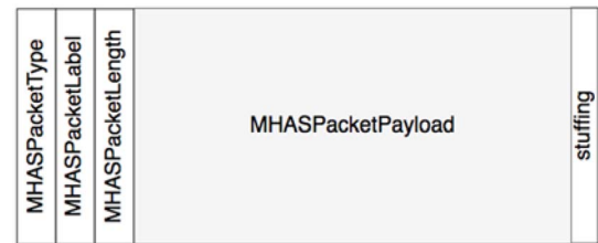
Fig. 31. MHAS packet structure.
