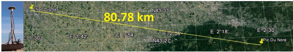
Fig. 13. Tests from ENAC roof antenna to the emitter of Pic de Nore.
