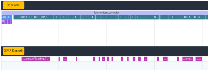
Fig. 3: A section of the trace collected of simpleFoam solver showing offloading of macro expressions, here TFOR_ALL_F_OP_F_OP_F in the momentum corrector stage, on MI300A.
