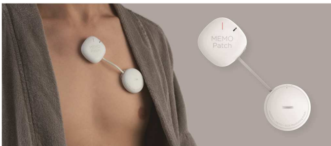
Figure 1. Patch-type ambulatory electrocardiograph, MEMO Patch, HUIINNO Co., Ltd.
