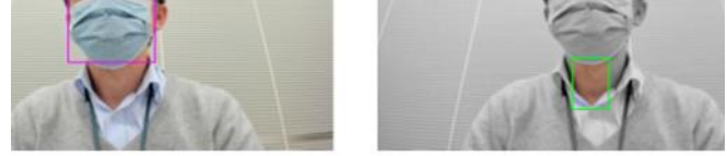
Fig. 4 Testing the ability of the newly developed prediction and prevention system to identify selected areas of the human body, namely the face and neck
