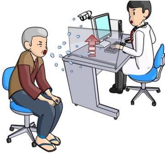
Fig. 3 As part of the newly developed prevention system (Jpn Pt. Appl. 2021-045978), this figure shows the use of a transparent partition actively blocking the airborne cough droplets.
