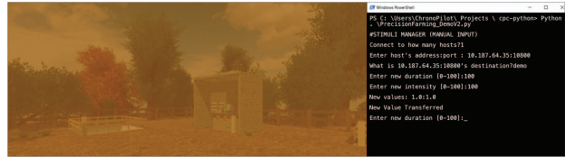
Figure 12: External VE control via example Python console application controlling a visual stimulus (golden flashing).
