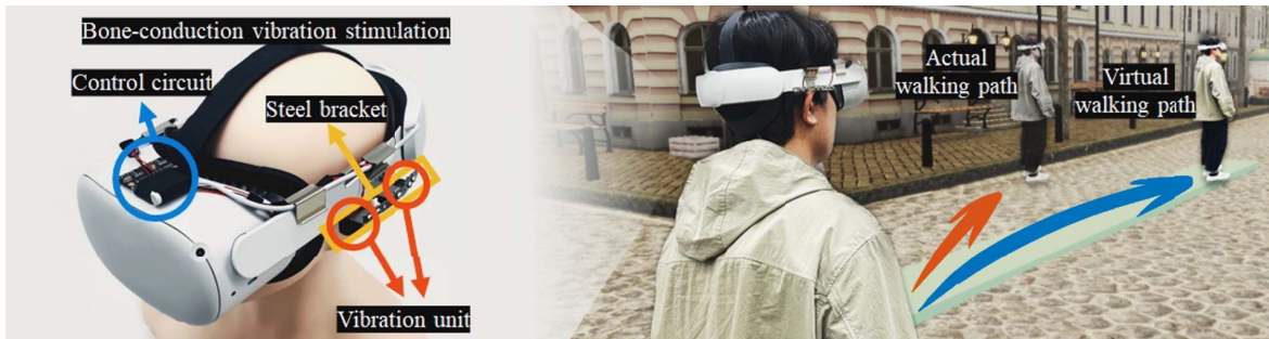
Figure 1: Conceptual illustration of the study: Utilizing bone conduction vibrations to enable users to seamlessly navigate without colliding into obstacles, thereby supporting uninterrupted walking.
