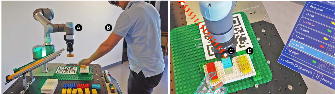
Figure 1: We present an AR-based assistant for collaboration in an assembly task between a (A) robot and (B) human operator in a joint workspace (left). We therefore present situated robot status information (e.g., movement path (C)) and task-related details (e.g., building instructions (D)) (right). Note: The path visualization and user's virtual hand are enhanced for better visibility in print.
