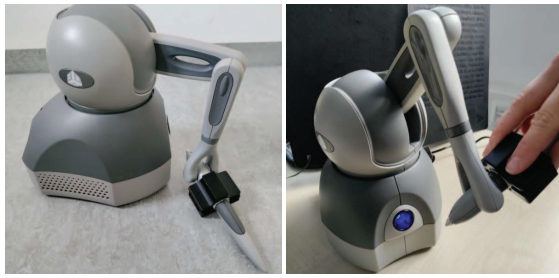
Figure 4: Geomagic Touch Device with a 3D printed attachment mimicking the US probe.
