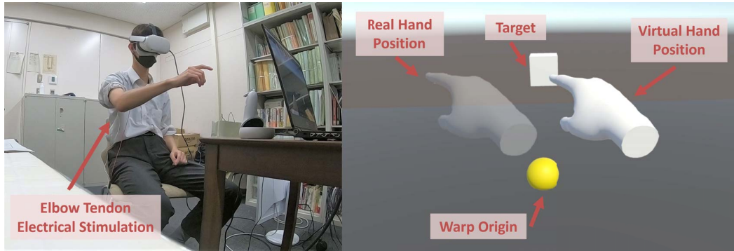
Figure 1: Hand redirection with noisy tendon electrical stimulation. Participants wore electrodes around the elbow of the right arm, and were exposed to weak, noisy electric stimulation during reaching tasks. In the virtual environment, each participant moved the tip of their index finger from the warp origin in front of them straight to the target at the back. Only the virtual hand, displaced from the actual hand position corresponding to the amount of movement, was visually presented.
