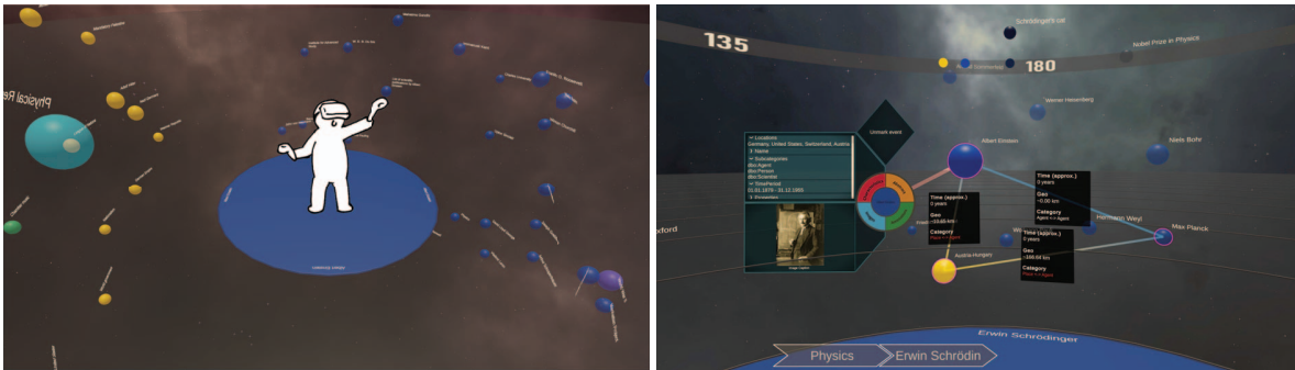
Figure 1: We present a tool for exploring historical data in VR using a head-mounted display. Left: The user is placed on a platform representing the main historical fragment (e.g., a person or an event) of their research (here Albert Einstein ). Other related fragments are represented as colored labeled spheres and are arranged around the user based on their historical interrelationships. Users can select a sphere to make it the new main fragment, thereby allowing for an immersive exploration of the dataset. Right: For every sphere, a detail window with more information on the corresponding fragment can be opened. An exploration history in the lower field of view shows the order of visited main fragments (here Physics and Erwin Schrödinger ). If a sphere is marked, a corresponding mark appears on a compass view in the upper field of view (e.g., a blue mark for Albert Einstein ). The relation details , here shown for Albert Einstein , Austria-Hungary , and Max Planck , reveal additional details about their historical connections.
