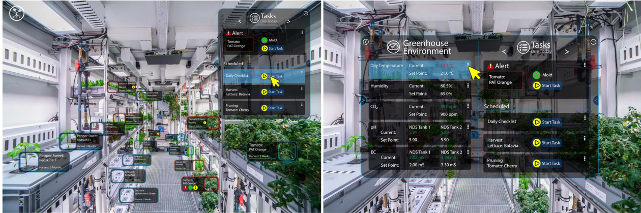
Figure 2: Concept of the ARCHIE 2 AR interface: Exemplary user view on the AR headset showing the scheduled tasks and plants inside the EDEN ISS greenhouse augmented with labels visualizing plant-specific information (left); Greenhouse Environment submenu (right). The yellow mouse pointer only illustrates a selection action on the interface (not part of the prototype). [17]
