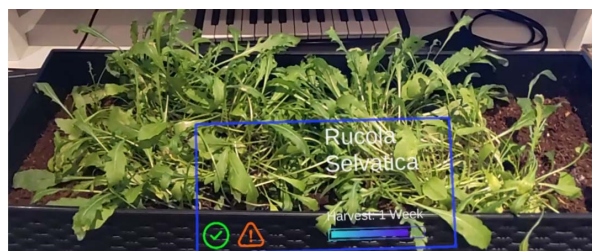
Figure 5: Augmentation label of the AR interface for the detected arugula selvatica plants with information on the name of the plant, the duration until harvest and icons to draw attention to status messages. The label is visualized on the ARCHIE 2 AR interface. [65]
