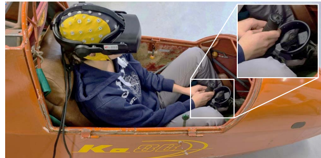
Figure 2: Participant using the control stick of the glider, to which an HMD controller was attached.
