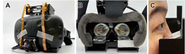
Figure 3: Prototype HMD. A) Front view, B) Back view. The white part of the right eye is the sponge between the face and the HMD. The sponge in the left eye area is removed for the photo, C) Bottom display placement relative to the face.
