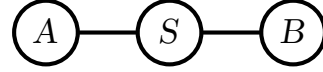
Fig. 4. Choice of qubit order for the implementation of the circuit on a QPU.
