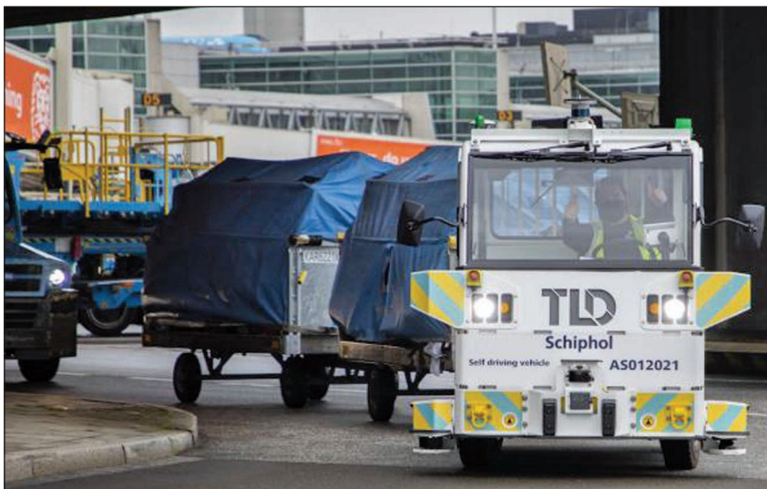
FIGURE 1 Look! No hands!!! Testing autonomous baggage tractor. (Source: TractEasy with EasyMile's autonomous technology at Schiphol airport.)
