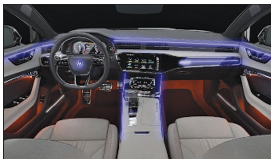
FIGURE 3 The light bar with multichannel RGB LEDs. (Source: Melexis; used with permission.)
