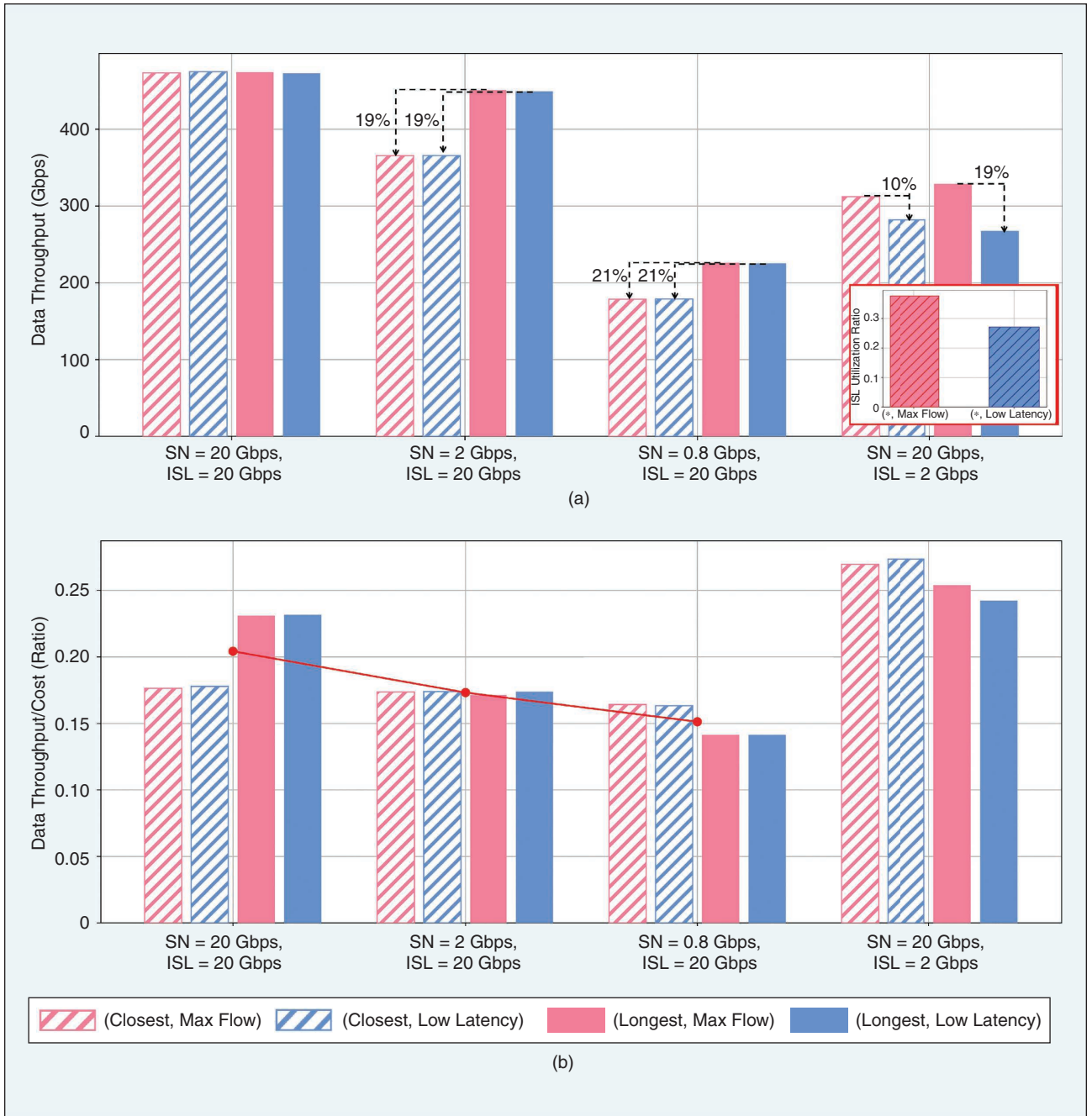
FIGURE 5 Simulation results of (a) data throughput and (b) its ratio to cost. Gbps: gigabits/s.
